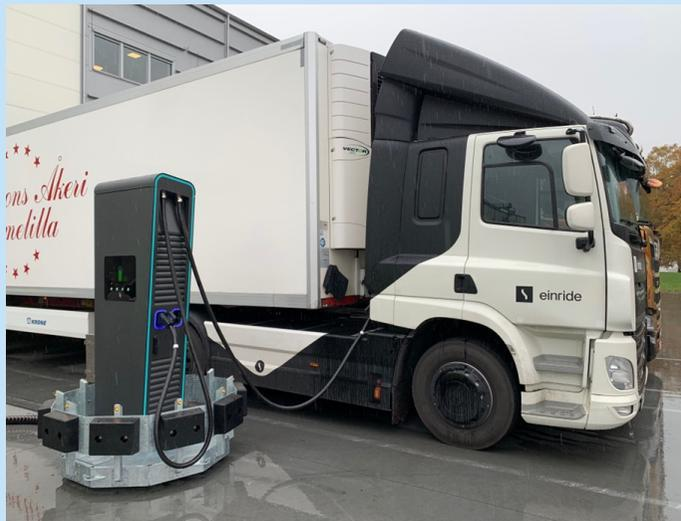
On the sides of the platform bumpers are placed in the same height as the bumpers on the trucks. This means that if a truck hits the platform the two parts will simply just bump away from each other. The energy supply for the charger was made flexible meaning that if a truck hits the charger, they could just use a forklift to get it back into place. See the picture below for the example.
