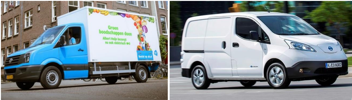
Figure 2-1 Examples of N1 category electric vehicles. Source: Albert Heijn (left), Nissan (right).
